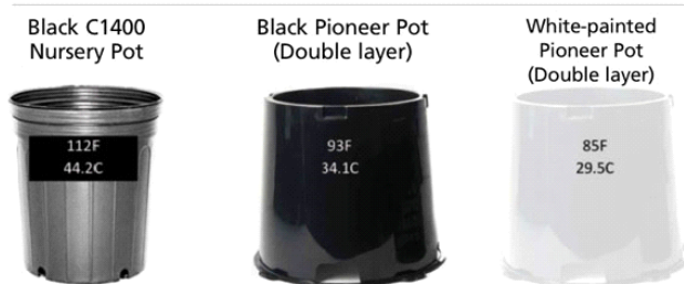
Figure 2. Substrate temperatures inside three types of container: a black nursery pot, a black Pioneer pot that has a double layer (insulation) and evaporative cooling in the inner layer, and a white-painted Pioneer pot, which also reflects radiation. Temperature was measured on the south side of the pot between substrate and plastic wall at 4-in. (10-cm) depth on a warm and sunny Florida day (89F/31.7C) air temperature with an average 1,773 micromol-m -2 s -1 of photosynthetically active radiation.
