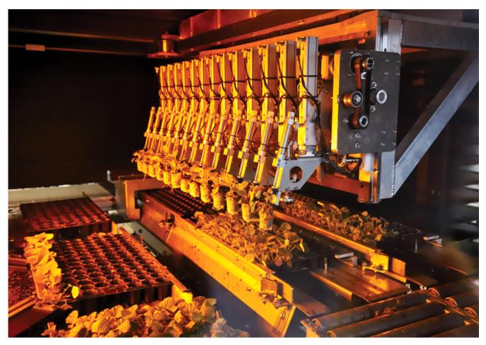
There's nothing new (at least in high-tech greenhouses) about using cameras and computers to grade and sort plugs and cuttings. What is new is analyzing pictures of the root zone, as well as the green portion of the plant, as is happening in this photo of a new Young Plant Sorter from Dutch equipment specialist Flier Systems (represented by AgriNomix in North America). *GrowerTalks* saw it in action in November at perennial liner grower Gebr. Alkemade in Lisse, the Netherlands.
