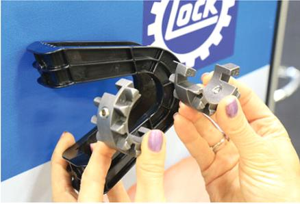
Another is the EZD 52, a unique two-piece pinion that allows for easy fitting and retrofitting onto a shaft without having to slide it on from the end, making it super easy to replace a defective pinion. The innovation won two different awards in Germany, including one from the Federal Ministry of Food & Agriculture.
