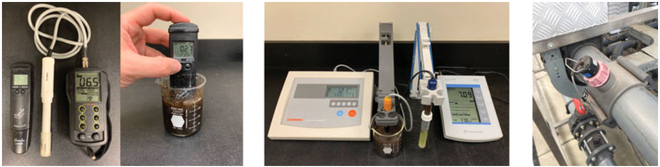
Figure 1. Hand-held and portable meters that measure both pH and EC (left). Using a hand-held pH/EC meter to conduct a 2:1 soil test (right).
