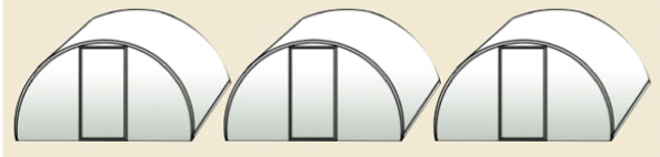
Figure 1. Increasing the footprint efficiency of a 10-acre greenhouse by 2% is equivalent to adding three 30-ft. by 100-ft. greenhouses.
