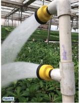
As can be seen in Figure 3, if two shut-offs are used, the cone of water can be controlled with more efficiency. Different nozzles can be used depending on the size of water cone required. If the shut-off close to the nozzle is fully open, then it will deliver the liquid with the designed accuracy. The other shut-off can control the water pressure and maybe the main tap can be modified so that the hosepipe is easier to move around.
