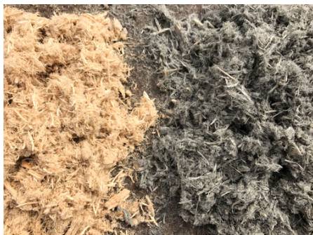
Figure 4. Coloring of wood fiber (with charcoal) is easily done during the mechanical processing of wood chips.
