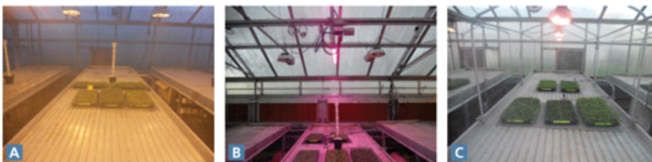
Figure 2. A) Examples of high-pressure sodium (HPS), B) light-emitting diode (LED) Top lighting and C) photoperiod treatments (wire mesh was used to reduce light intensity).
