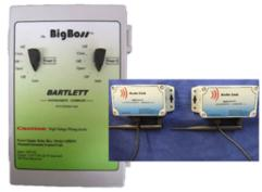
The Big Boss from Bartlett Instrument is a 24VDC power supply designed to control two 10A motors for rolling up/down walls. It can be used manually as an independent unit or it can be linked to one of their controllers for automation. The Big Boss also has 10A resettable circuit breakers to protect each motor and the 5A circuit breaker protects it from power surges and shorts. It retails for \$465.00.
