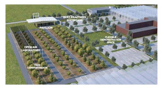
The facility will include an Open Air Laboratory that has individual tree compartments, each with their own integrated sensor technology to recreate conditions faced by trees in urban settings while recording responses to stress and monitoring weather, soil function and canopy health. This is the first of its kind in Canada. Phase one will have 36 compartments, but they plan to expand that to 80.
