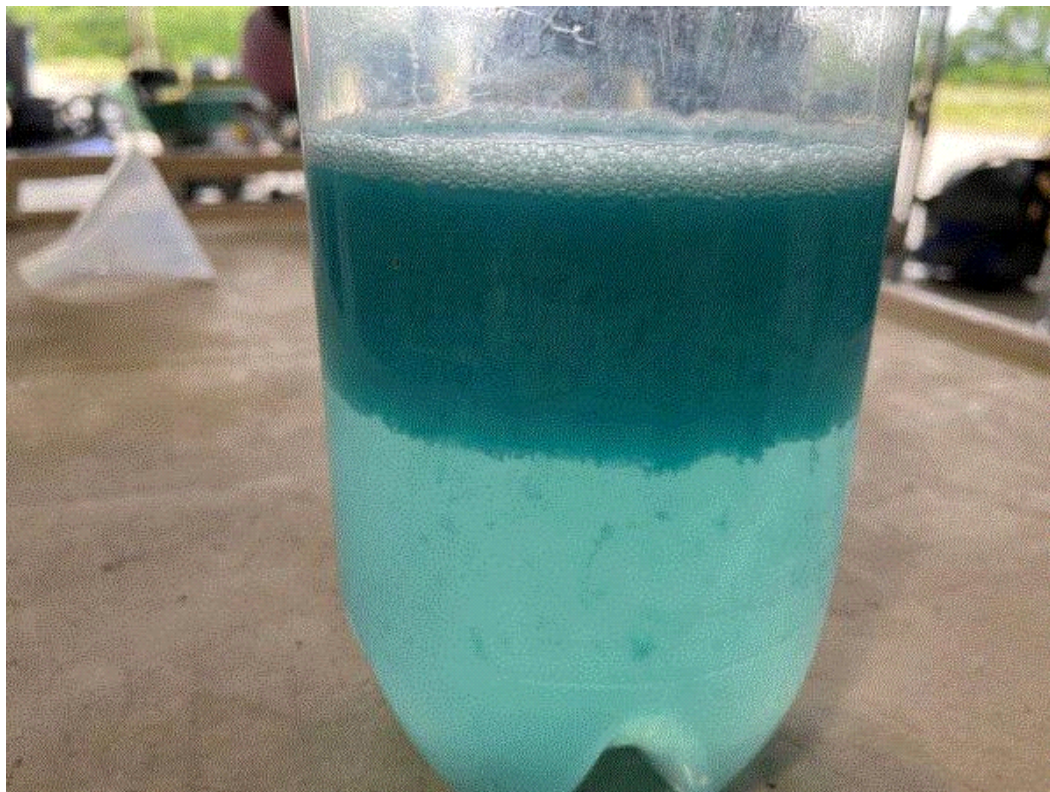
Want to know what happens when you mix mefenoxam and a copper fungicide? Behold! (Photo: Zach Small, SePRO.)
