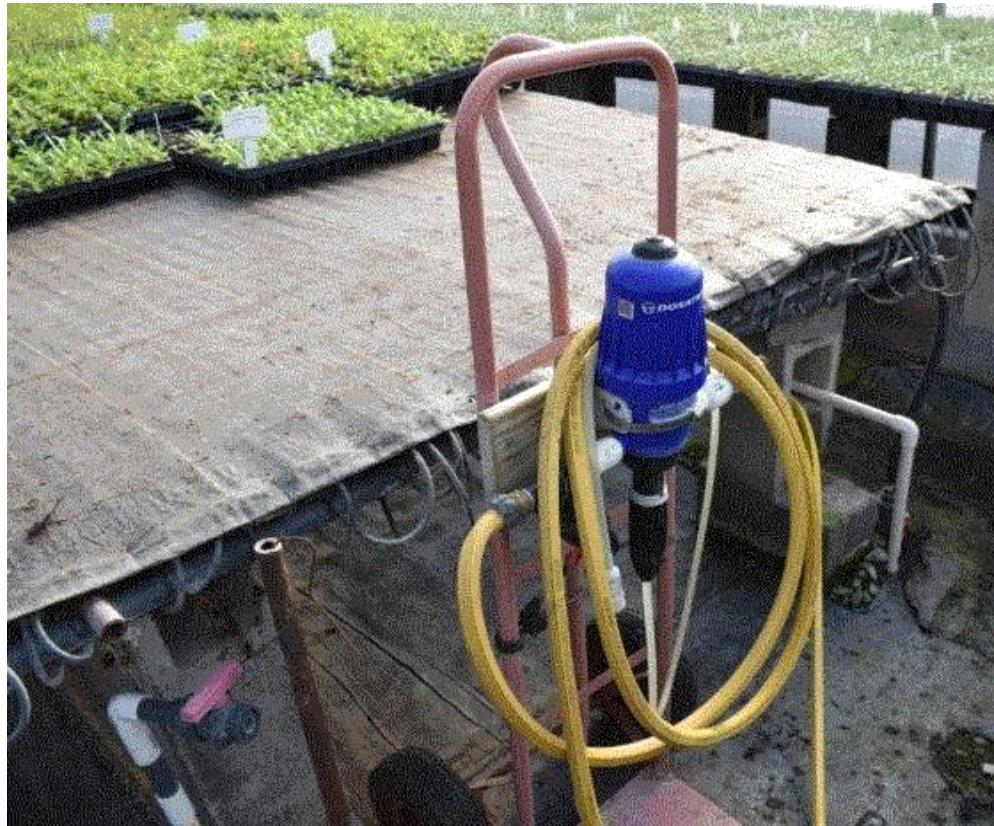
A calibration check is the easiest way to make sure your injector is hitting its mark. To do this, you'll need the injector (of course), an EC meter, your favorite fertilizer and a cup or beaker for sample collection.
