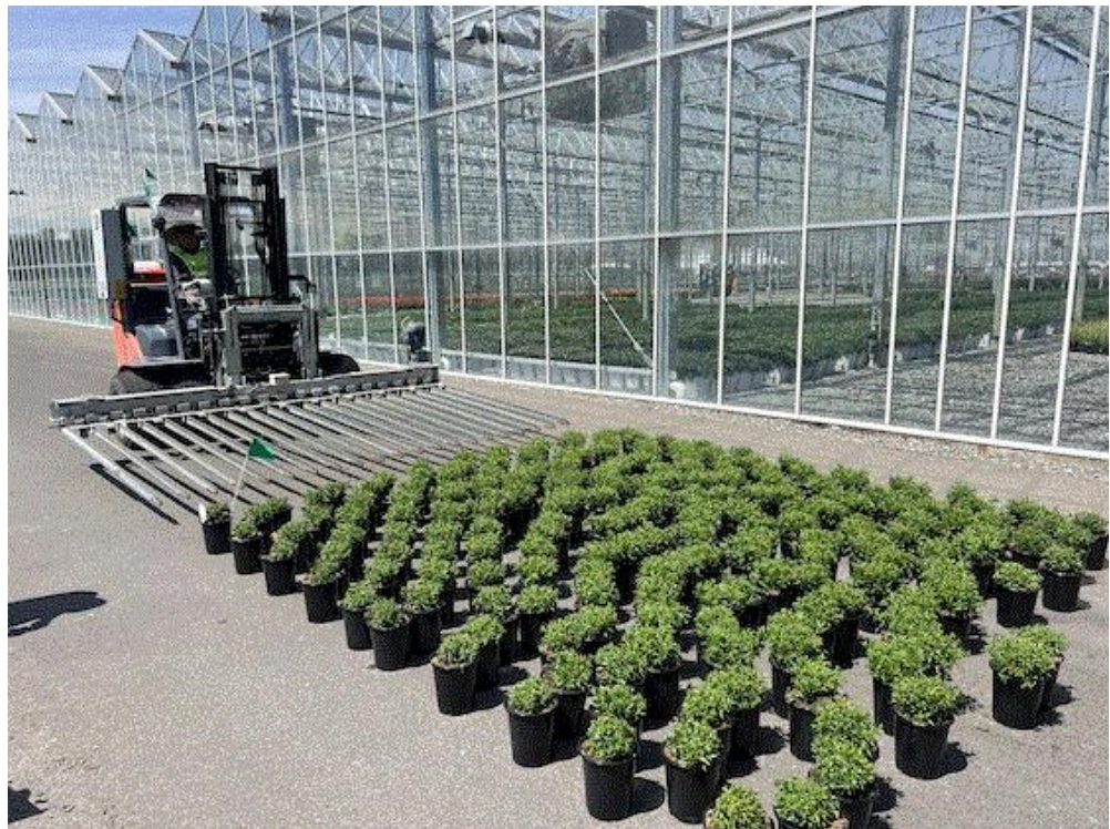
The single plant-spacing fork is extremely helpful during outdoor mum season when you're moving 50 acres of plants around like the folks at Smith are.
