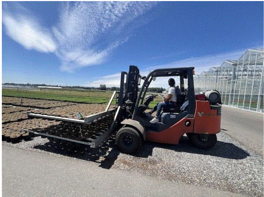
This is the plant-moving fork that has two levels to move twice as many pots.
