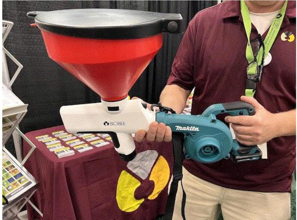
For just \$400, you can buy a powered applicator that cuts the time it takes to spread beneficial insects on an acre of crops from 1 hour to just 10 minutes—an 83% improvement!—and do it more gently and more evenly. **BugFlow**, from BioBee, is a battery-powered hopper (3-qt. capacity) that connects to an off-the-shelf battery-powered blower.
