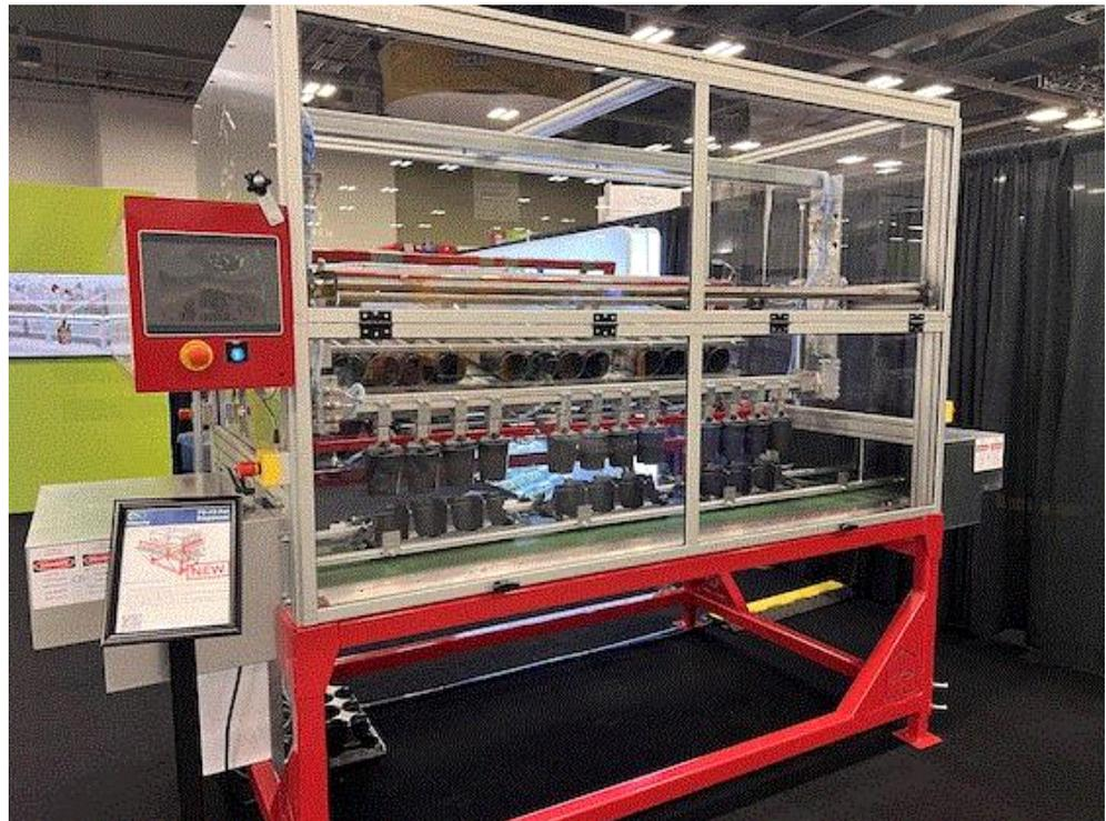
AdeptAg (formerly AgriNomix) has launched a new high-capacity pot dispenser that fills three shuttle
