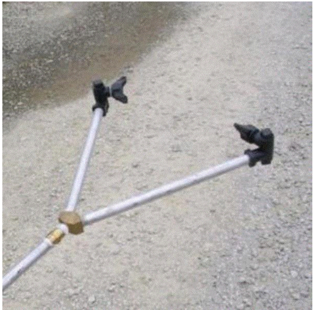
A modified spray wand like this directs good spray coverage to the trunk, which is the part of a tree that needs to be protected from ambrosia beetle. Go HERE for an article on the benefits of this spray wand compared to an airblast sprayer. (Photo credit: Steven Frank, NC State University.)
