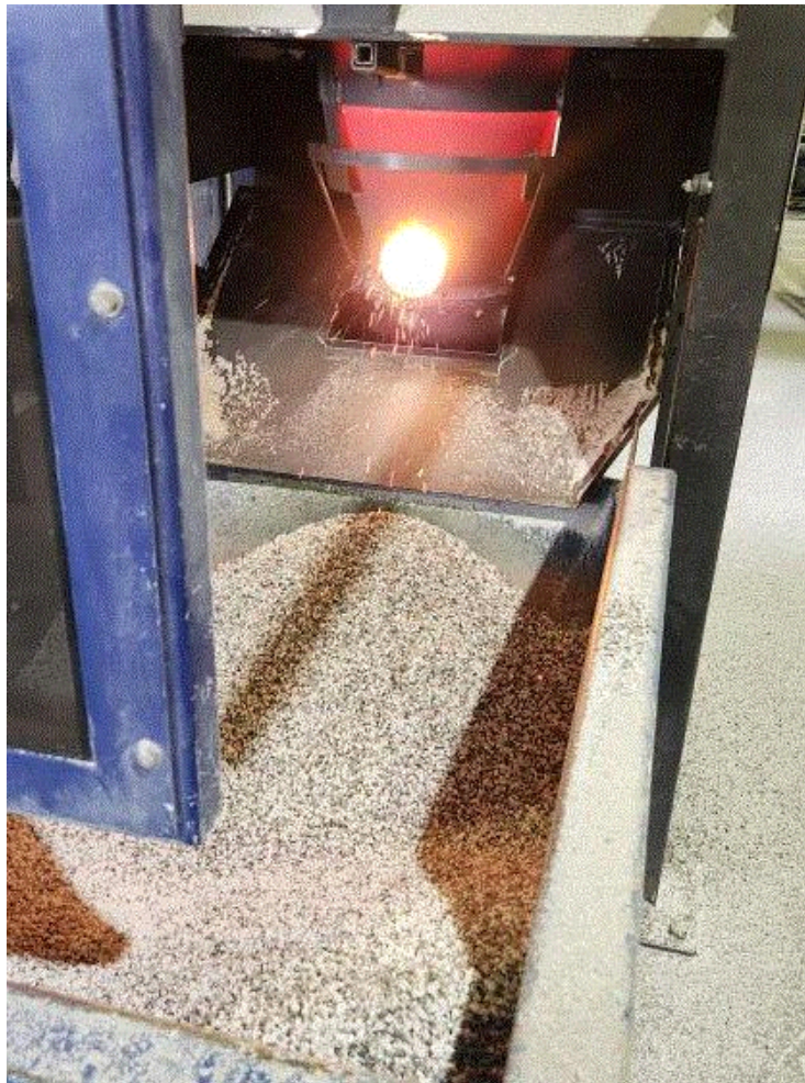
Perlite is expanded through very high heat. The individual particles are red-hot when they emerge!
