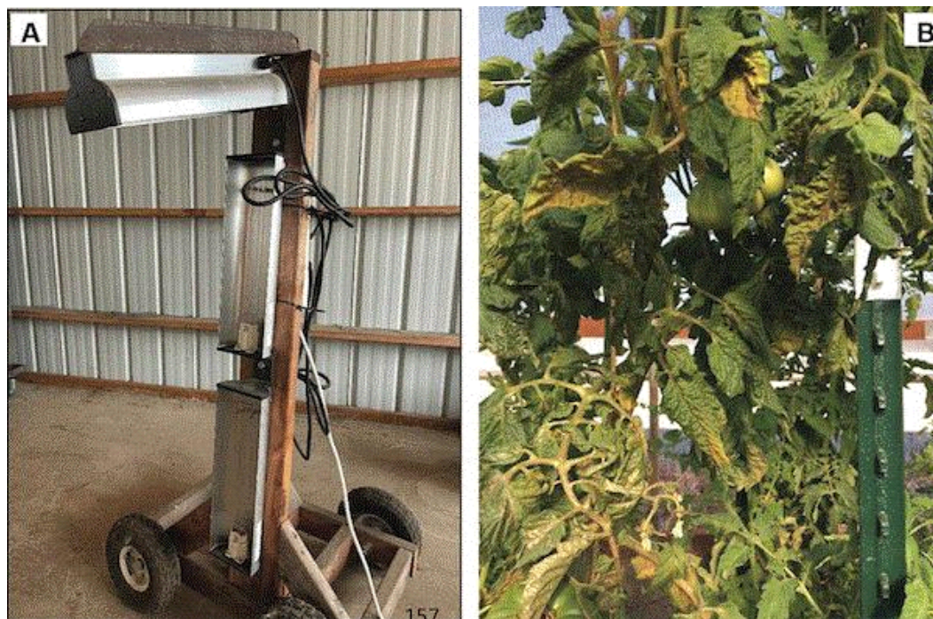
A) Hand-constructed stand cart (5-ft. tall) used for ultraviolet-C (UV-C) treatments. The cart contains three UV lights (2 ft. x 5 ft.; CleanLight XL) that produces broadband UV-C at 253.7 nm. The cart was placed next to and above individual tomato plants for treatment. B) Phytotoxicity on a tomato plant after receiving the first two treatments of UV-C light for 90 seconds per plant. (Photo credit: Buckland et al. 2023; HortTechnology 33, 2.)
