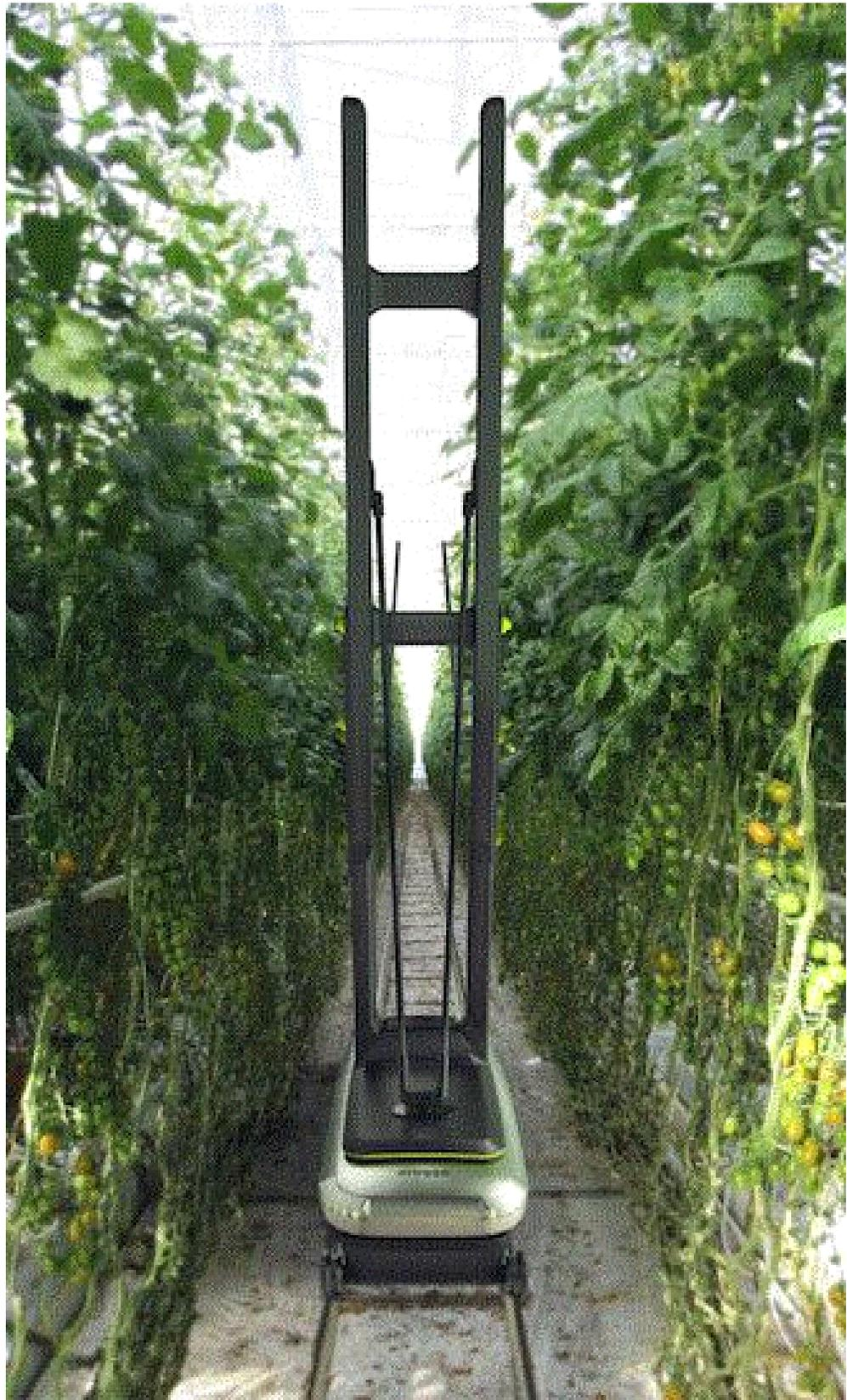
As you can see, it rolls along the same rails used by other internal transport systems commonly used in hydroponic greenhouses. Equipped with cameras and artificial intelligence-based computer vision, the robot recognizes flowers ready for pollination. An air-pressure mechanism then applies calibrated air pulses to the selected flower.
