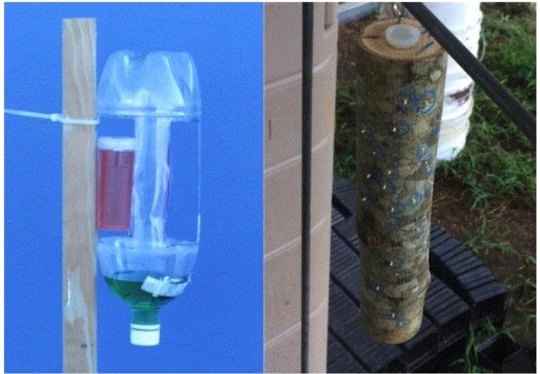
A soda bottle trap with ethanol lure (left; photo credit: JC Chong) and an ethanol-filled bolt trap (right; photo credit: Matthew Brown, Tennessee State University).
