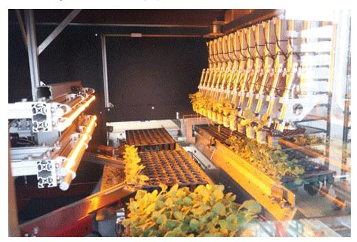
The machine's Aris cameras look at three things: The top of the plant (looking down), the side view of the plant, and the side view of the roots. The grower inputs how much of each they want,
