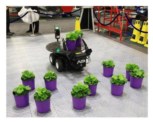
Also unlike Harvey, Big Top is modular. The base provides power, wheels and brain; the carrier and manipulation components can be changed out for various functions, such as pruning (which was on display, but not operating). They say they've got six more versions on the drawing board.
