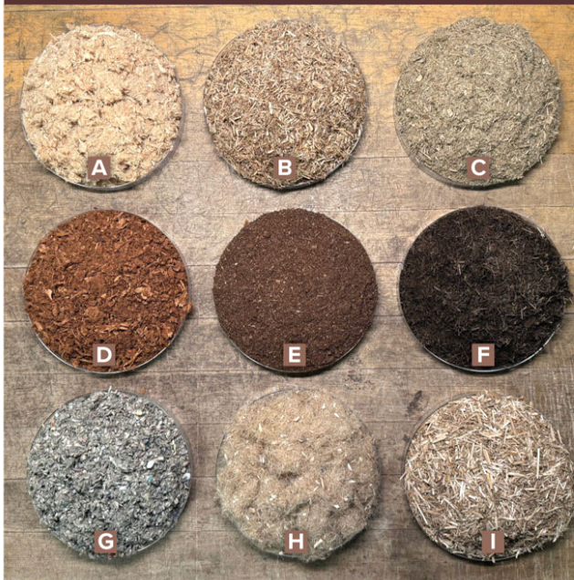
Figure 1: Some materials used with peat to formulate hybrid mixes include: A) conifer wood fiber; B) hardwood fiber; C) bamboo; D) extruded bark; E) double-processed bark; F) sugarcane bagasse; G) Pittmoss; H) kenaf fiber; and I) miscanthus.
