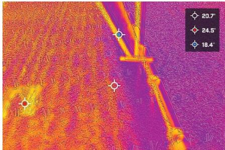
Accurate leaf temperature data can help growers improve mist control. When leaf temperature is available in real time, the timing and frequency of misting can be adjusted based on climate conditions. This allows the system to apply water based on VPD, rather than relying solely on a time clock. Basing misting frequency on climate can reduce unnecessary misting, reduce leaching and runoff, and minimize the risk of disease from excessive moisture.
