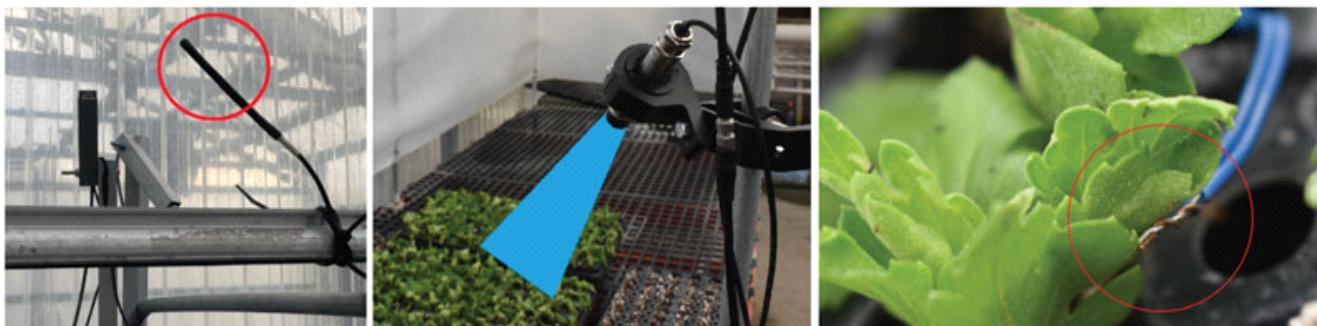
Left: Leaf temperature sensors, including (from left to right) an Artificial Leaf sensor (which is a thermistor above the mist zone exposed to sunlight), an IR sensor (which measures infrared thermal radiation emitted from the leaf and substrate surface) and a thin-wire Thermocouple (which is a sensor placed on or inside the leaf surface).
