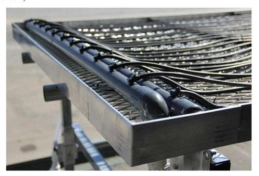
The new system from Stuppy is designed in-house with EPDM rubber tubing that resists high temperature or chemicals, while offering superior heat transfer capabilities and durable design. Mike says hydronic bench heat has been proven to promote higher seed germination rate,
