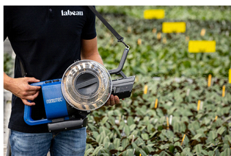
Figure 4. Aiobreez has a sealed compartment that holds up to 3 liters of material. The entire drum rotates at various speeds based on an easy-to-adjust dial on the top. This keeps the mites evenly blended, as well as controls the dosage of the application.
