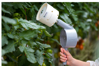
Figure 3. The rotating dispenser pot on the Airbug and Airobot line of blower units is critical to their success. This ensures that a uniform blend of mites and carrier fall into the airstream for dispersal at all times.
