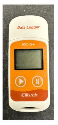
Pictured: Data loggers work by using built-in sensors to measure environmental conditions, such as temperature and humidity, at regular intervals. The device collects and stores this data in its memory, which can later be accessed via software or a connected device like a computer or smartphone.
