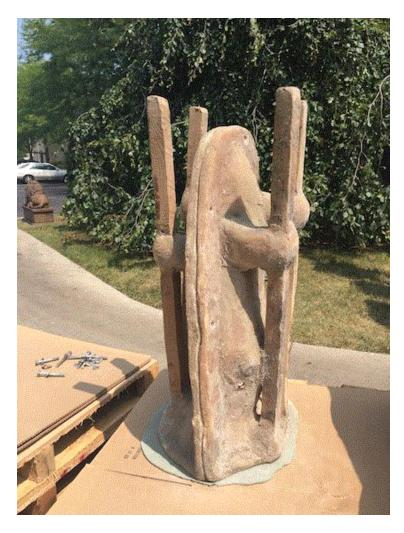
... which is filled with a simple slurry of limestone, sand and good-ol' Lake Michigan water. It cures for a day, the mold is removed and then it goes through a staining process.
