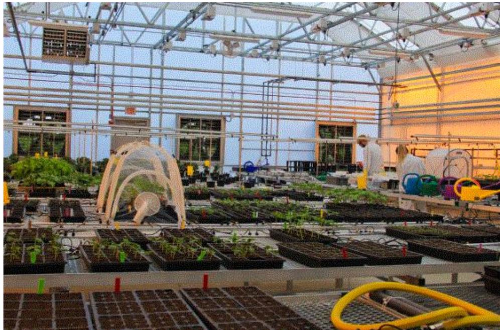
Valent built four research greenhouses to help their scientists simulate field growing conditions, complete with an automated climate-control system, on-bench heating and ebb-and-flood hydroponic capabilities. Now they can grow from the young plant stage to when the plant is close to harvest. They can have up to 10 experiments going on in one bay.
