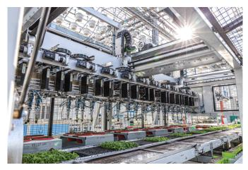
The Pic-O-Mat is linked to a pot destacker, pot filler and table loader, all of which communicate with each other. Select a new pot size program on the transplanter and the destacker, filler and loader automatically change to the new pot size, too. In fact, you can control the whole line from any one of three control panels. To make it easy for workers who may speak multiple languages, any problems and where to locate them, are shown in 3 -D graphics on the screens.
