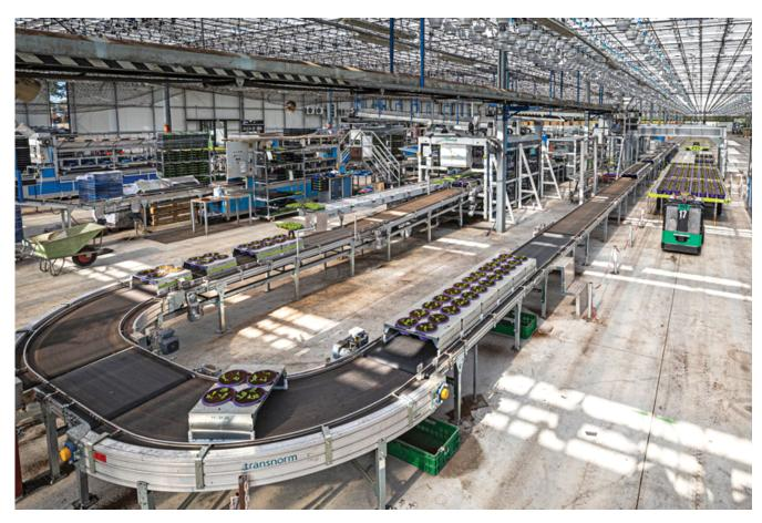
When you have to fill (and refill) more than 100 acres of greenhouses with bedding plants, how can you be both fast and flexible? This new transplant-ing line is the solution at Dutch greenhouse Kwekerij Wouters, one of the largest potted and bedding plant operations in Europe.
