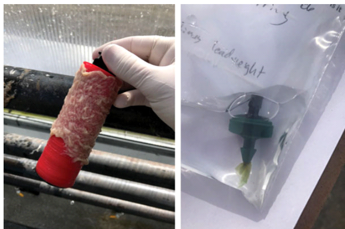
Figure 3a and 3b. Examples of microbial biofilm on irrigation systems.
