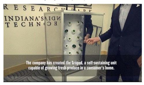
The appliance is called the Gropod, a "self-sustainable refrigerator-sized unit capable of growing fresh produce in a consumer's home," according to a release from Purdue University. The system uses advanced algorithms that make it aware of the types of plants inside and how to grow them.
