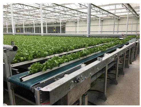
The Green Automation hydroponic NFT growing system is fully automated, from medium filling and seeding to harvesting. The lettuce is moved automatically through the greenhouse during the entire growing process. Pictured: Conveyor belts transporting the lettuce to the harvesting station.
