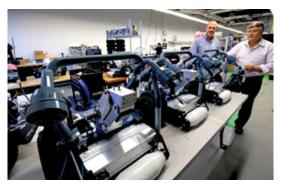
Harveys number HAI-1245, 1246 and 1247 await final assembly by Don Haras (right), manufacturing test engineer at the Harvest Automation facility in Billerica, Massachusetts. That's CEO John Kawola looking on. "Harvey" is the pet name for Harvest's HV-100 plant moving robot. Launched just two years ago, there are now some 150 HV-100s at work at 27 nurseries and greenhouses across the country.
