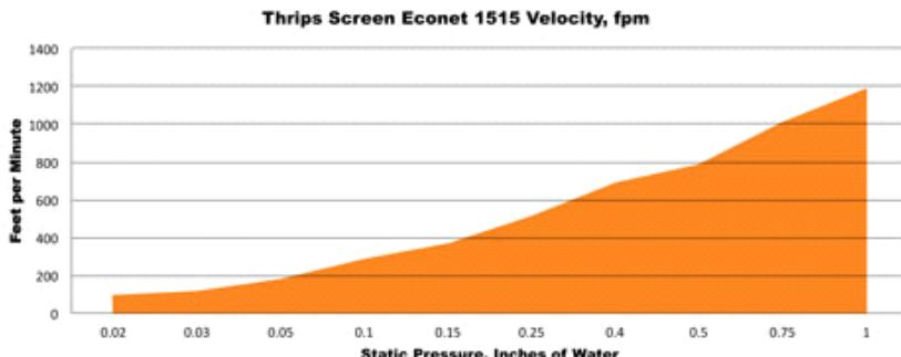
each insect screen. Pressure-velocity curves are developed by evaluating insect screens in a wind tunnel.
