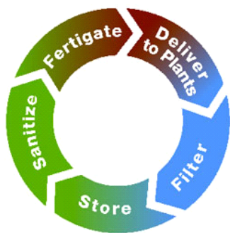
Figure 2: Basic flow diagram of sub-irrigation system water cycle.
