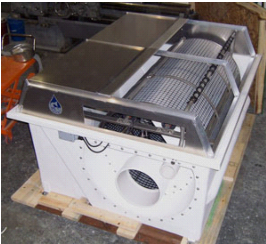
View of a fiberglass-enclosed drum filter.
