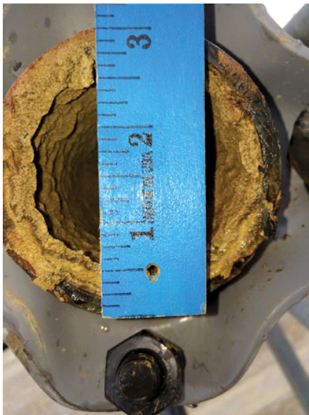
Figure 2. Iron precipitates on a main irrigation pipe.
