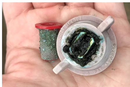
Figure 1. Emitter clogged on the outside with algae and on the inside filter with chemical precipitates.
