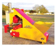
The first machine of this type—that does four different jobs—is compact, so it fits almost anywhere. There are dual soil returns in the conveyor belt so that the soil stays in the machine instead of spilling
