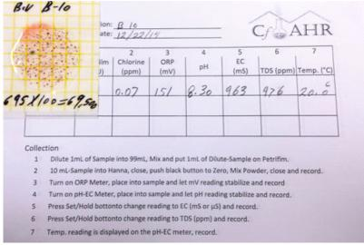
On-site water quality monitoring by a grower to determine efficacy of disinfestation process. Chemical water quality was assessed with pH, electrical conductivity and oxidation reduction potential (ORP). Biological water quality was assessed using methods developed for irrigation monitoring with Petrifilm aerobic count plates (3M).
